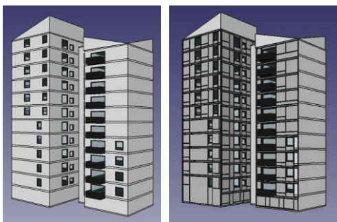
Figure 3. Left, Demo Building model in Milan. Right, building in Milan with added prefabricated façade with solar panels (ENSNARE project)
